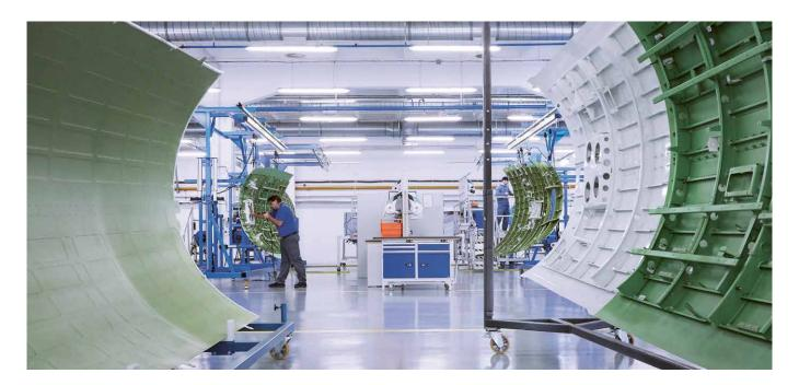
The Aerostructures business division develops, produces and installs structural parts for aeroplanes, in particular complete fuselage sections and components for wings and control surfaces. RUAG Aerostructures
