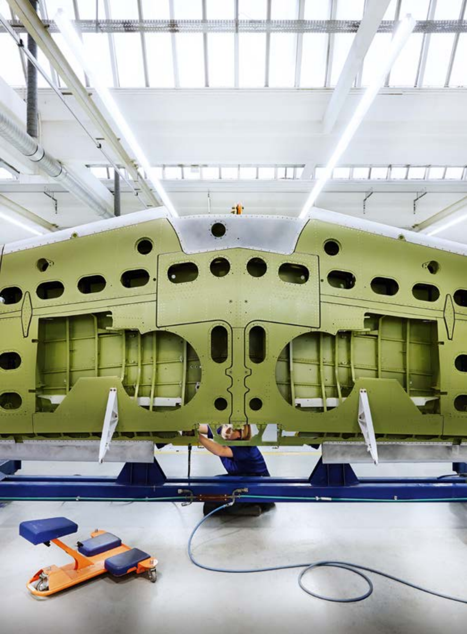
Final inspection and preparation for final acceptance of a Pilatus PC-21 wing structure at the Emmen site.
