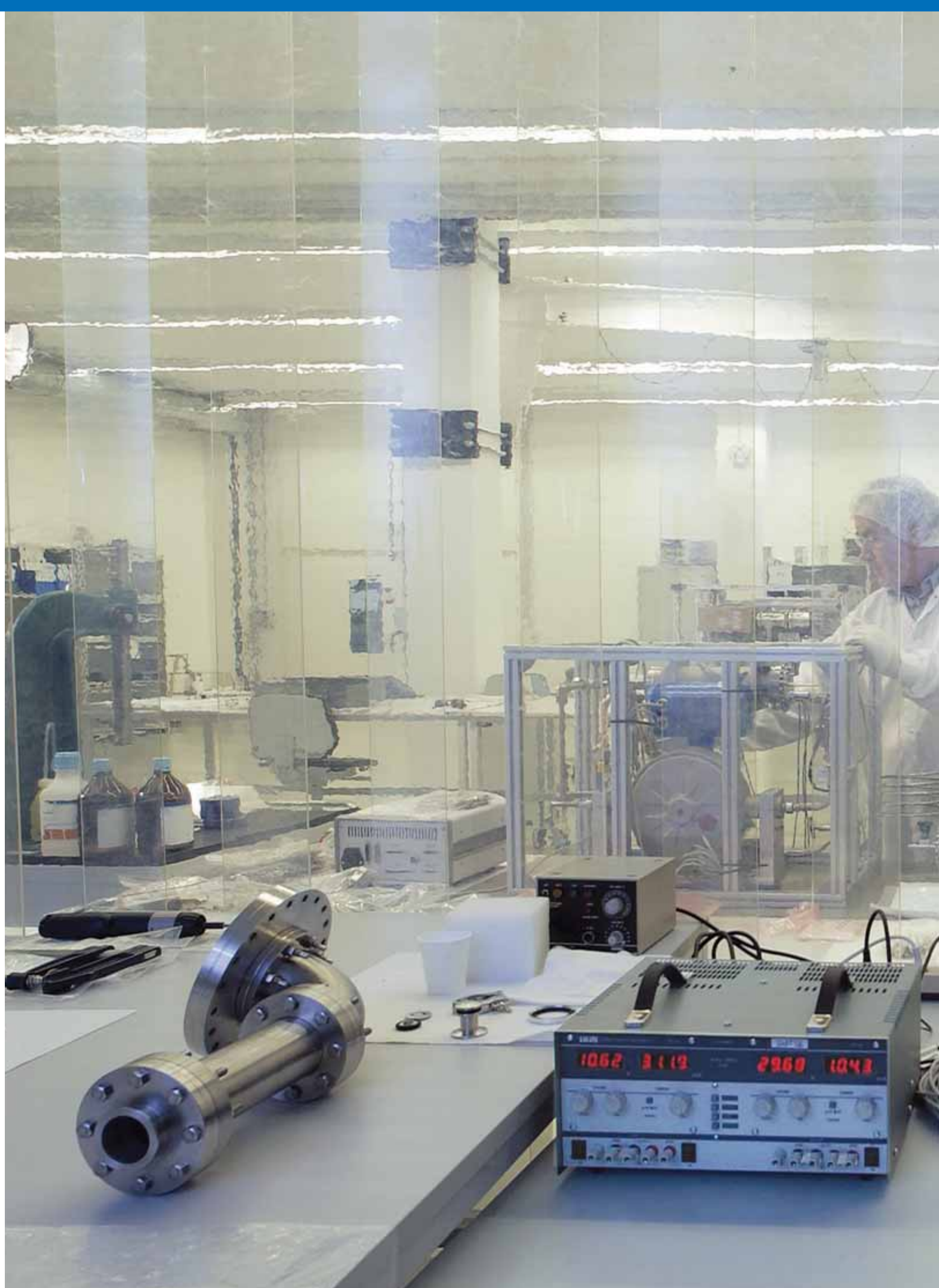
Work in progress in the clean room on the vacuum gas sub-system for the international space station's materials research laboratory
