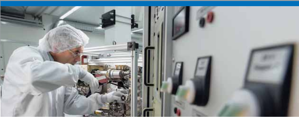
Test rig for ammonium/water pump in satellite cooling circuits
