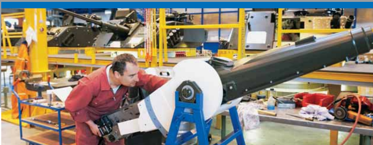
Pre-assembly of the gun for the new Armoured Infantry Fighting Vehicle
